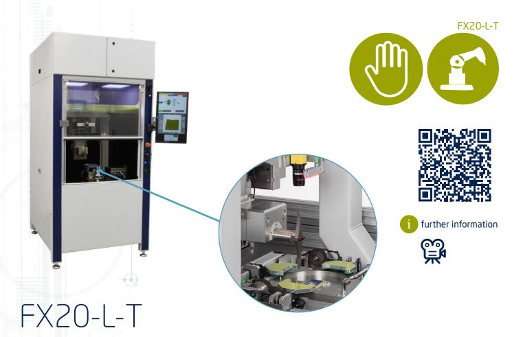
The FX20-L-T is an automated ultrasonic welding machine for production. It is suitable for welding power electronic modules (e.g. IGBT modules) or cell contacting systems (battery applications). The machine is available with a pattern recognition system for checking and correcting the welding position and particle cleaning system.
